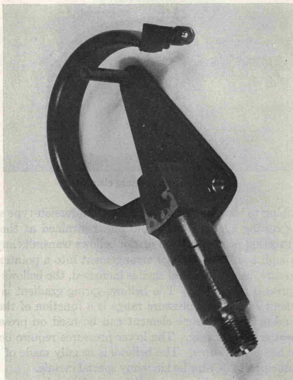
Fig. 6. "C"-type bourdon tube pressure element.
